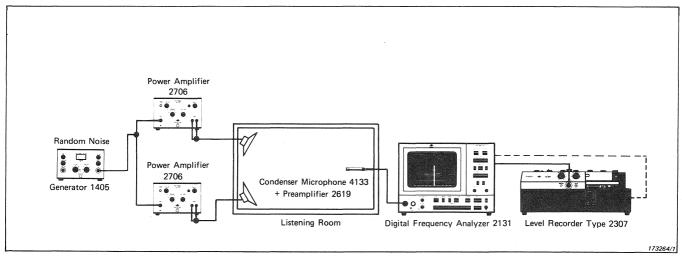
Fig.10. Measuring set-up with "pink" noise 20 Hz to 20 kHz. The result is immediately read out on the screen
