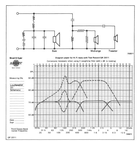
Fig.23. The corrected cross-over network and the corresponding curves
